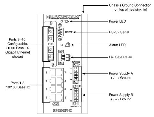
Figure 1.1. RS900GP Front Panel
